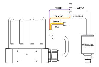
Figure 31: Two Wire Transducer Wiring
