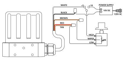
Figure 22: Potentiometer Analog Setpoint
