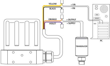
Figure 35: Monitor 4–20 mA External Feedback (Ground Referenced Input)
