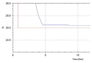
**Figure 59: Typical Tuning: Checking for Offset at Setpoint 1** As was true for Setpoint 2, some offset correction will be required at Setpoint 1.
