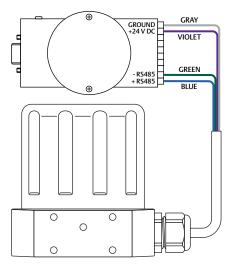
Figure 27: RS485 Connection (RS232 to RS485 Converter)
