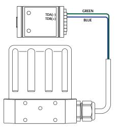
Figure 28: RS485 Connection (USB to RS485 Converter)
