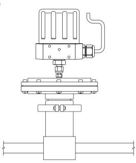
Figure 8: Mount the ER5000 on the Regulator
