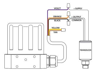
Figure 32: Three Wire Transducer Wiring
