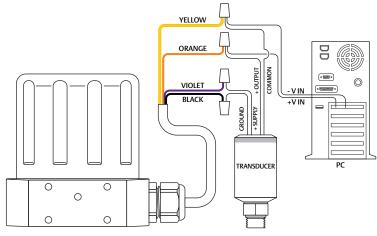
Figure 38: Four Wire Transducer, Monitor Voltage Produced by 4–20 mA Feedback
