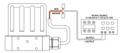
Figure 23: Current/Voltage Analog Setpoint
