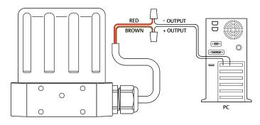
Figure 25: Active PC or PLC D/A Card Analog Setpoint
