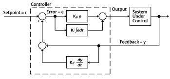
Figure 2: Simplified PID Control System
