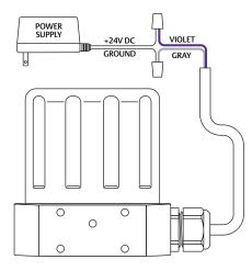
Figure 21: Wiring to 24V DC Power Supply
