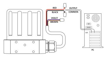
Figure 24: Passive PC or PLC D/A Card Analog Setpoint
