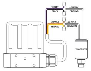
Figure 33: Four Wire Transducer Wiring
