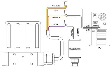
Figure 36: Two Wire Transducer, Monitor Voltage Produced by 4–20 mA Feedback
