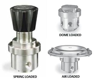
TESCOM 44-4600 Series is an extremely sensitive, high purity, single-stage regulator for specialty, flammable and industrial gases for low pressure and sub-atmospheric pressure control. Diffusion-resistant metal diaphragm seal ensures gas purity and leak integrity.
